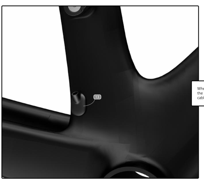
When using an electronic drive train, use the grommet (13) to fix the front derailleur cable.
