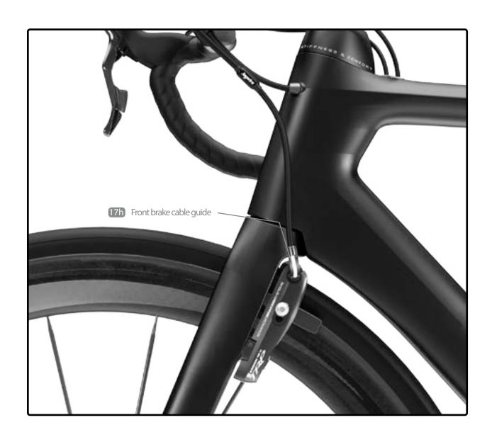
Note: The front brake cable guide (17h) should be front-oriented to ensure good rotation of the handle bar.
