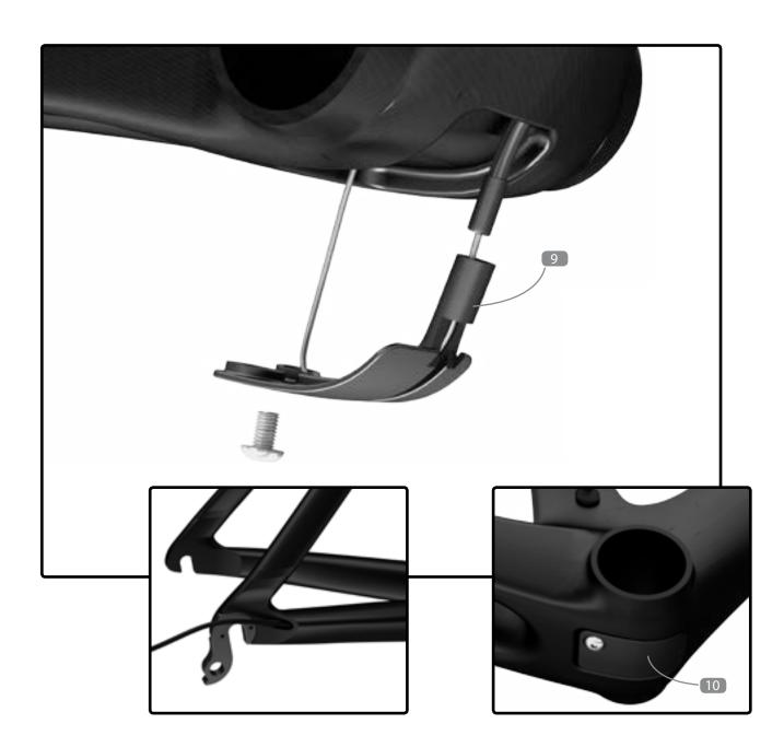
It's better to install the cable housing before installing the bottom bracket, crank and fork.
